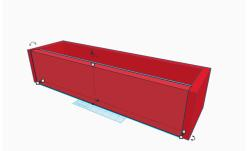
4. Attach the front piece with glue and decking screws (pre-drill the holes).
