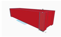
5. Attach the vertical pieces of trim on the corners with finish nails and glue.
